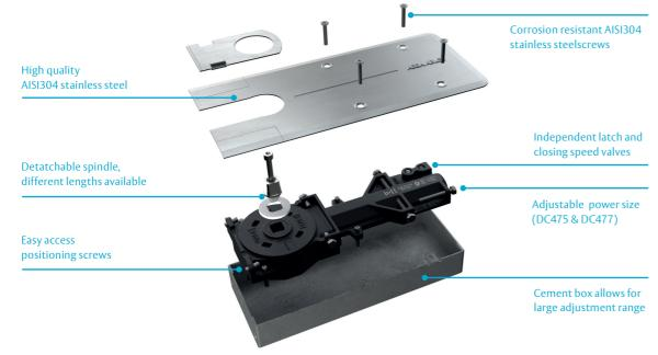
An ASSA ABLOY Floor Spring does its hard work completely out of sight, so your door remains the main attraction. All building users will see is a high quality stainless steel cover plate
