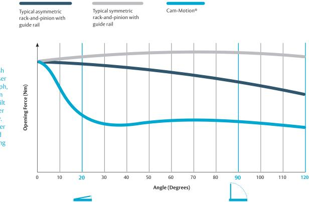
When you open a door equipped with a Cam-Motion<sup>®</sup> door closer from ASSA ABLOY, the force needed to open the door falls quickly.
