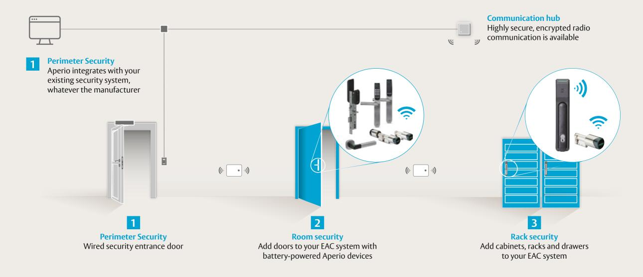
Keep your current EAC system and add wireless access control to doors and server racks with Aperio locking devices
